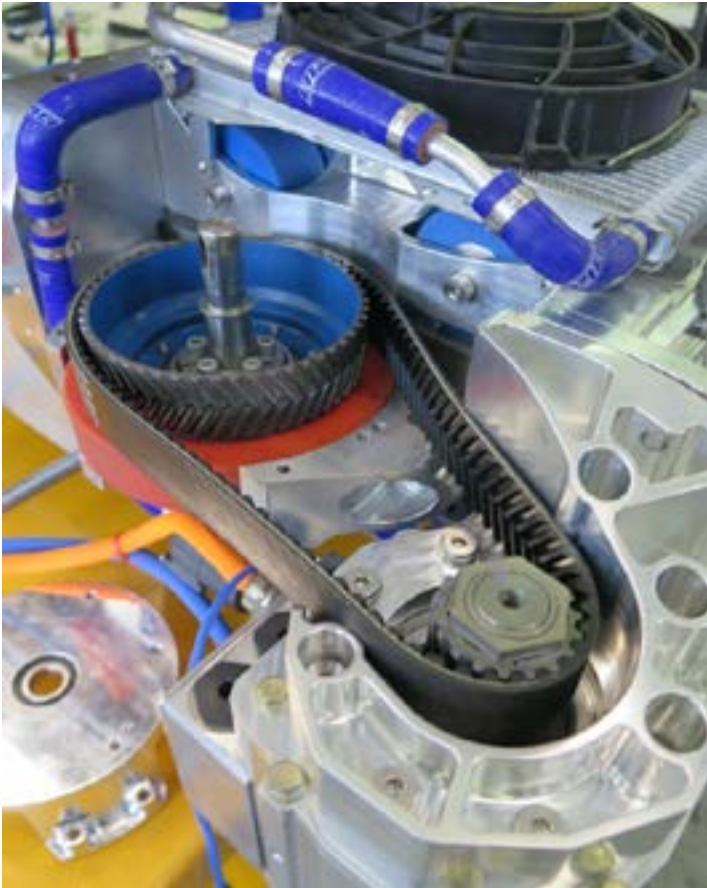
Double Helical high-performance synchronous belts for extra-quiet operation. Custom lightened sprocket and minimum bore pinion design
