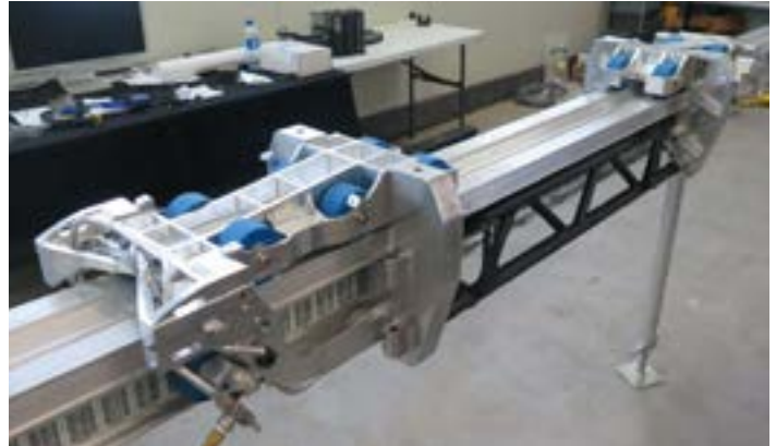
Bogies connected by 4043 tubular frame weldments
